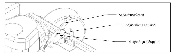
Figure 9: Securing Crank While Not In Use
